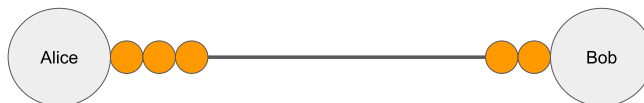
Fig. 1. A channel with capacity 5 and balances 3 and 2 for Alice and Bob, respectively.
