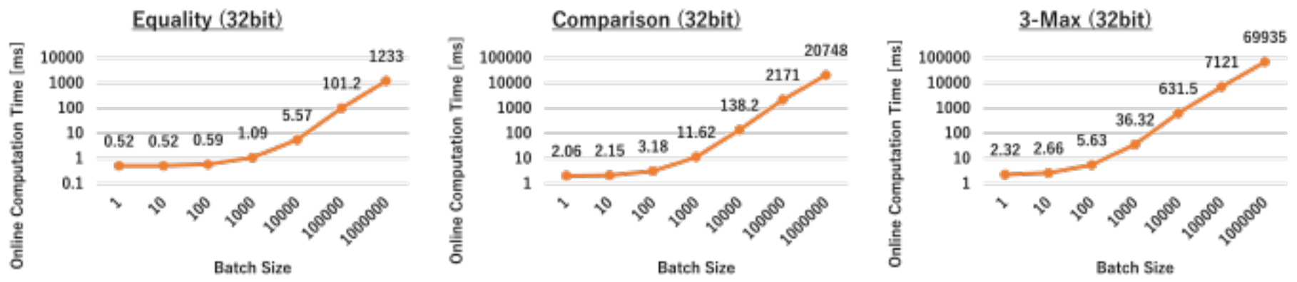
Fig. 2. Relations between batch size and online computation/execution time of the protocols over \mathbb{Z}_{2^{32}} .
